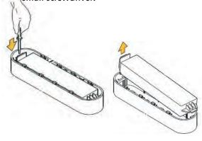
2. Install 2AAA alkaline batteries (included). Make sure the red light blinks. If red light does not blink, check batteries for correct polarity.
